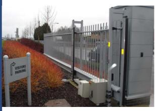
Eagle can supply cantilever sliding gates up to a clear opening of 8.0m. Typically the height of the gate is 2.4m but with our in house design team a system can be designed unique to your requirements.
